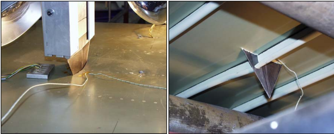
Figure 2: Standard-GLARE ® panel impacted under tensile load
