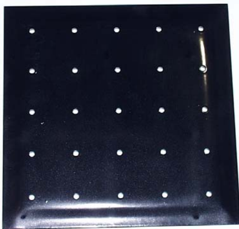
Figure 4: Outdoor weight gain specimens 4 , painted (P) and painted and drilled (PH) specimen
